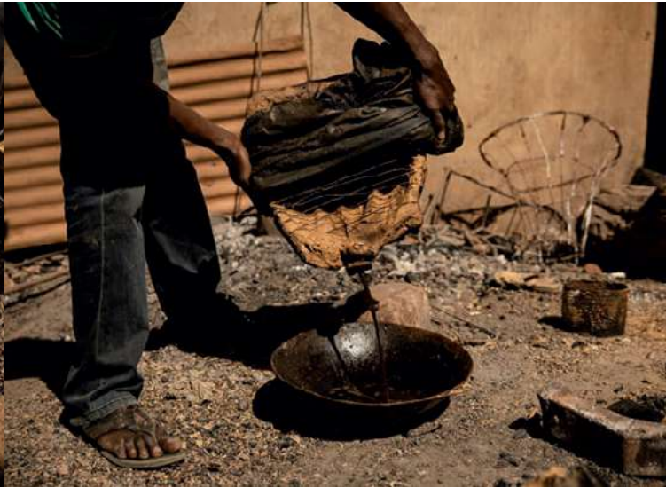
2. Once the clay has hardened and the wax melted, metalsmith Alidou Zoungrana drains the melted wax into a bowl, for reuse
