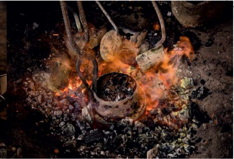
4. The recycled metal for the lamp is melted at 1,200°C over the outdoor fire
