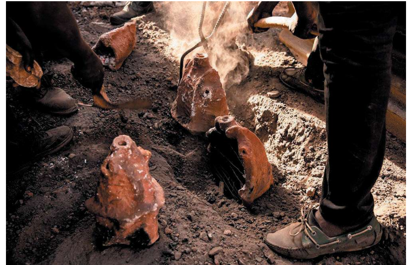
Top, the molten metal is poured into the hollow clay mould, filling the space left by the beeswax model. Bottom, the metal is left to cool and harden in the clay moulds for about an hour and a half. Photography: Sophie Garcia
