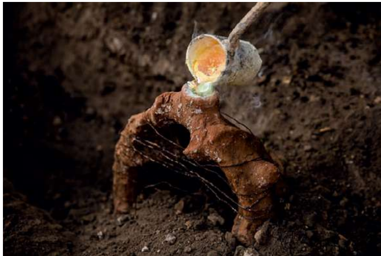
5. The molten metal is poured into the hollow clay mould, filling the space left by the beeswax model
