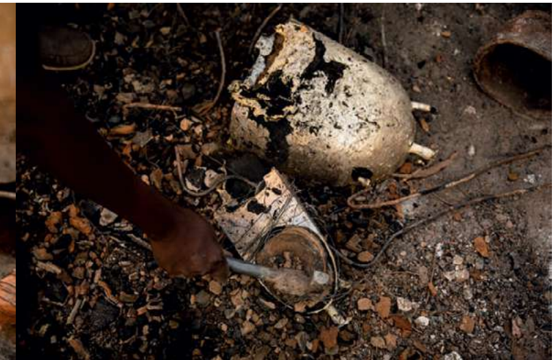
8. The clay layers are cleaned away to reveal the lamp's metal shells, which will be polished with a metal file for a smooth finish
