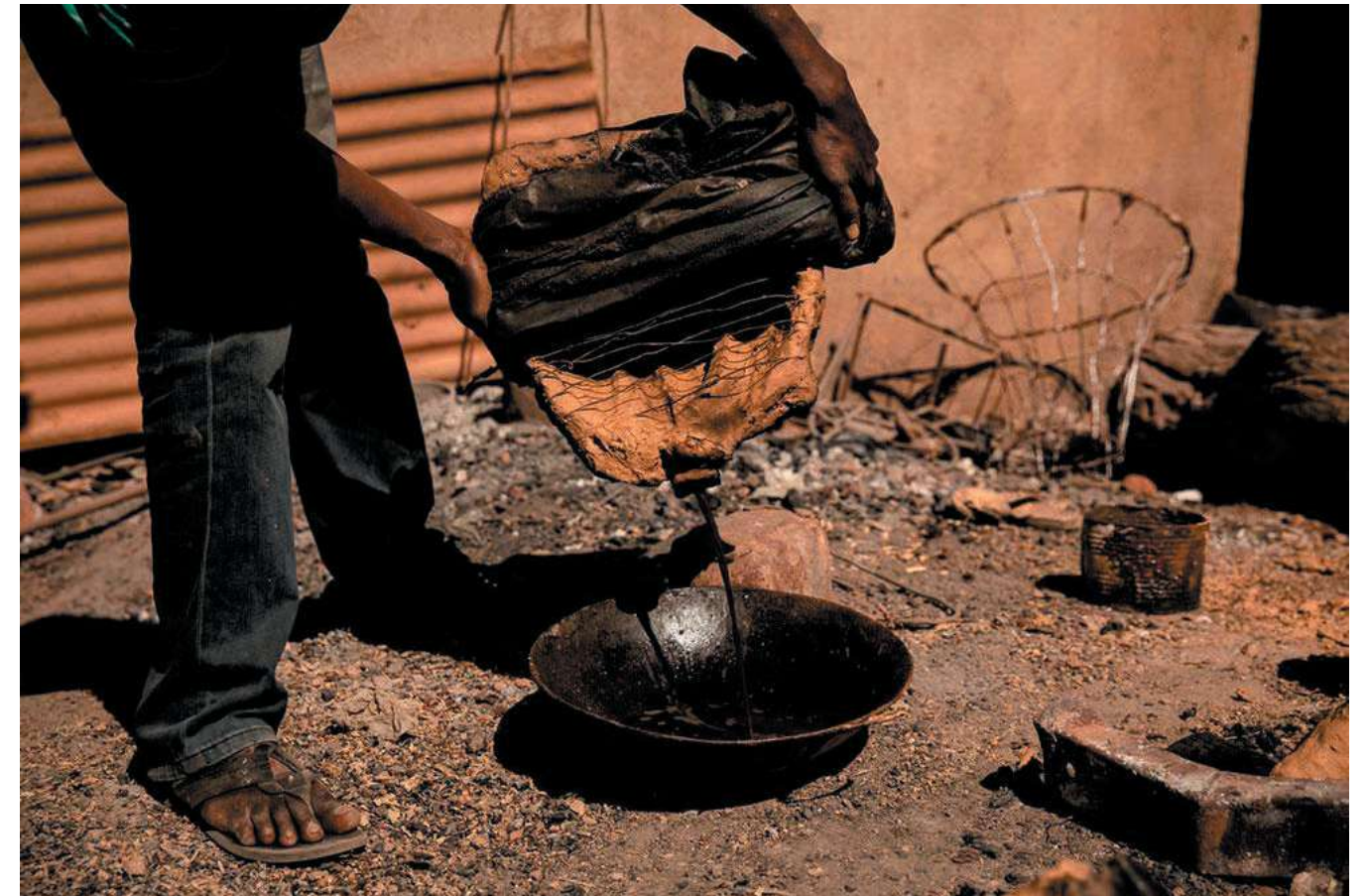
Top, a beeswax model of the lamp is wrapped in a mix of clay and horse dung, secured with metal wires, and baked for a few hours. Bottom, once the clay has hardened and the wax melted, metalsmith Alidou Zoungrana drains the melted wax into a bowl, for reuse. Photography: Sophie Garcia
