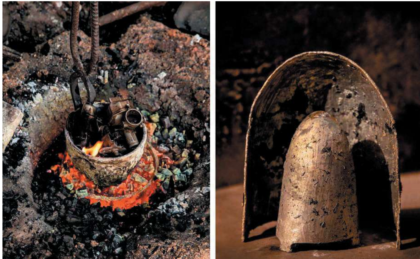
Left, recycled metal is melted down to create the 'Echo' lamp at a workshop in Ouagadougou, Burkina Faso. Right, the design before it is polished. It comprises two bronze curved forms that appear to cradle each other. Photography: Sophie Garcia
