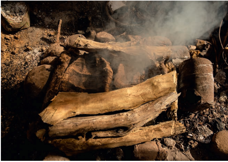
1. A beeswax model of the lamp is wrapped in a mix of clay and horse dung, secured with metal wires, and baked for a few hours
