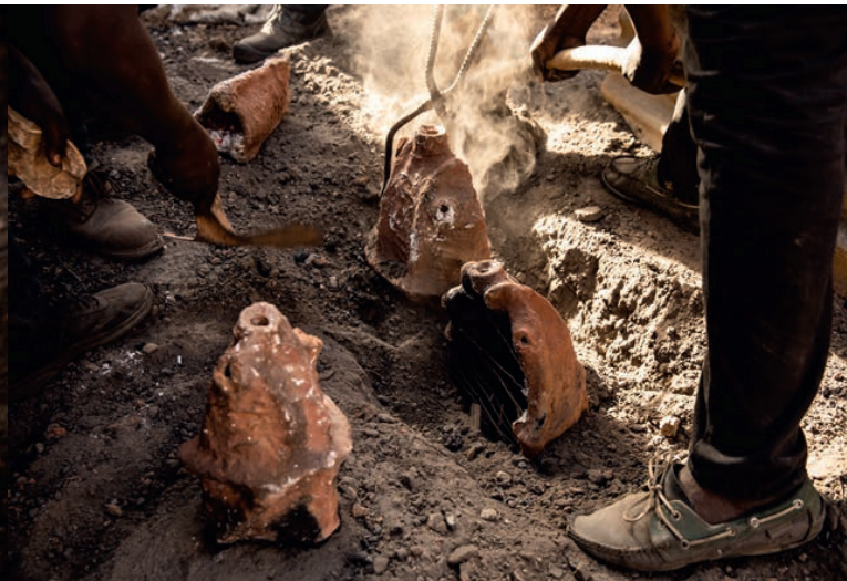
6. The metal is left to cool and harden in the clay moulds for about an hour and a half
