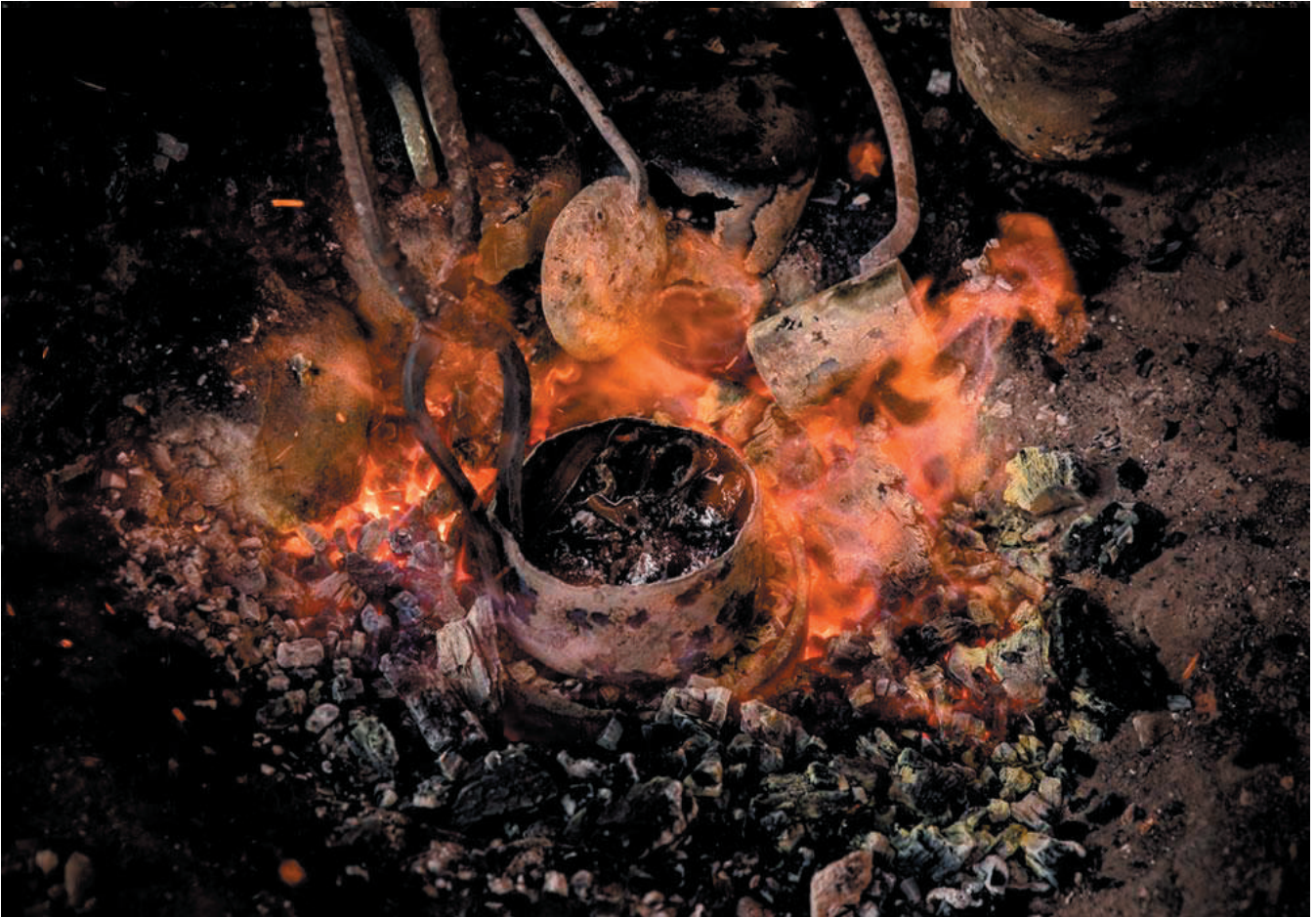
Top, metalsmiths Ousmane Koita and Denis Kabre remove the melting pot to add fuel to the fire while Roger Kabre observes. Bottom, the recycled metal for the lamp is melted at 1,200°C over the outdoor fire. Photography: Sophie Garcia
