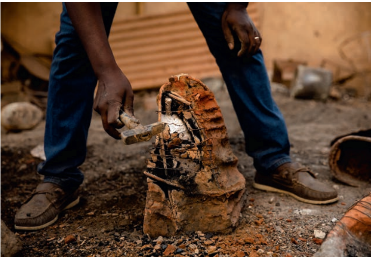
7. Denis Kabre breaks open one of the clay moulds, before removing the wires that kept it together
