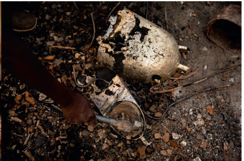
8. The clay layers are cleaned away to reveal the lamp's metal shells, which will be polished with a metal file for a smooth finish
