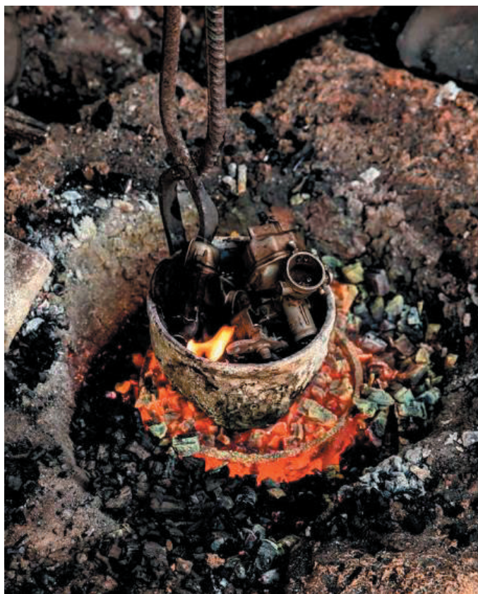
Left, recycled metal is melted down to create the 'Echo' lamp at a workshop in Ouagadougou, Burkina Faso. Right, the design before it is polished. It comprises two bronze curved forms that appear to cradle each other. Photography: Sophie Garcia
