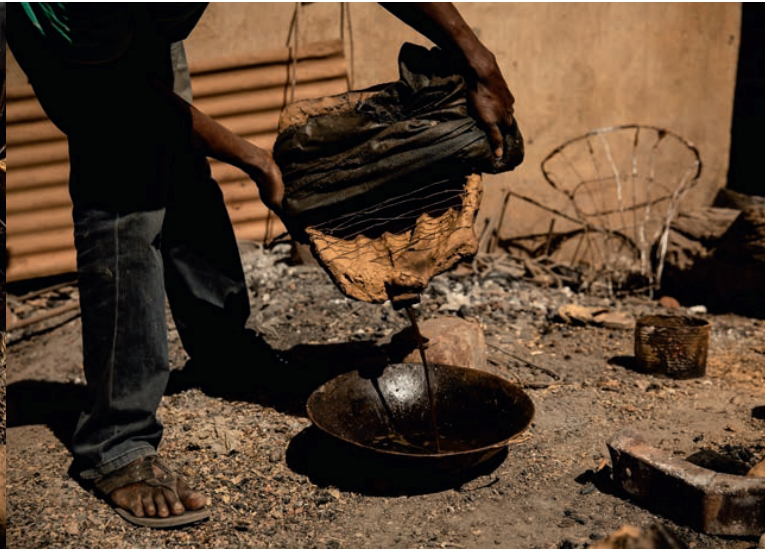
2. Once the clay has hardened and the wax melted, metalsmith Alidou Zoungrana drains the melted wax into a bowl, for reuse
