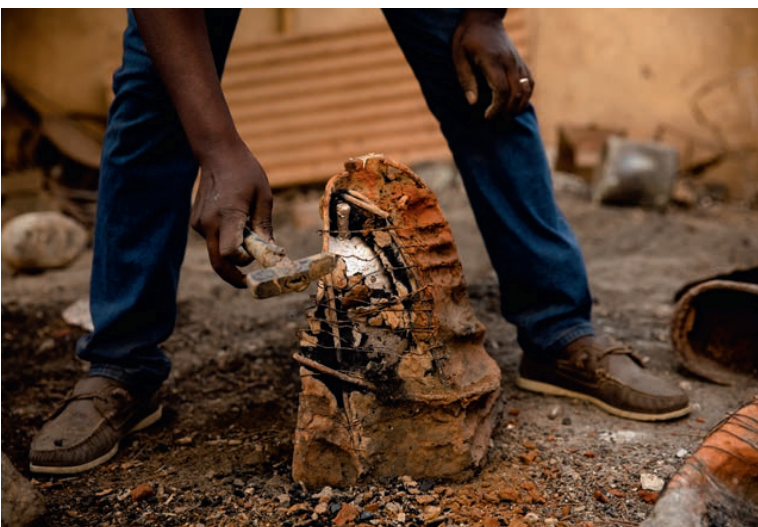
7. Denis Kabre breaks open one of the clay moulds, before removing the wires that keep it together
