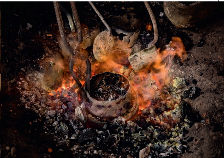
4. The recycled metal for the lamp is melted at 1,200°C over the outdoor fire
