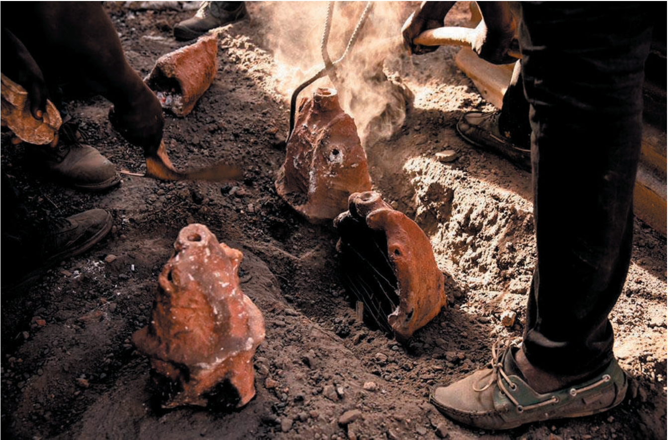
Top, the molten metal is poured into the hollow clay mould, filling the space left by the beeswax model. Bottom, the metal is left to cool and harden in the clay moulds for about an hour and a half. Photography: Sophie Garcia
