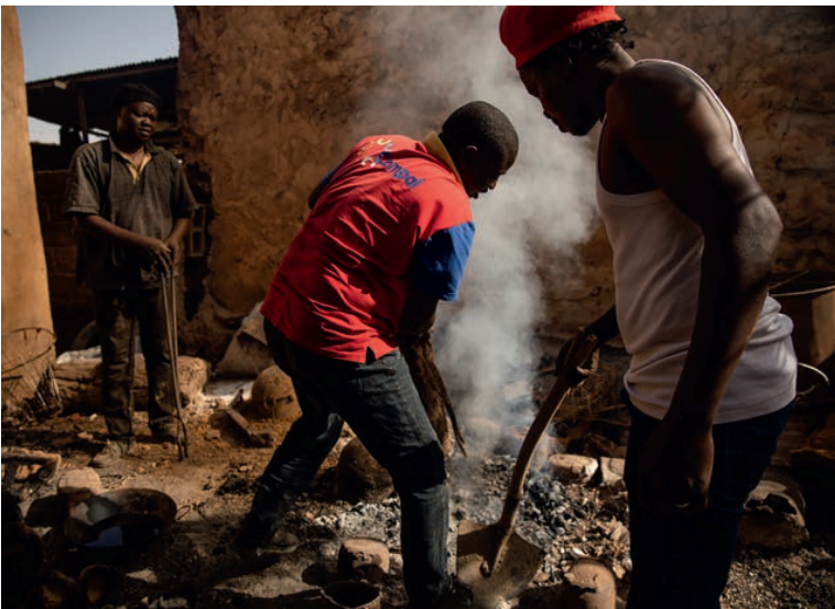
3. Metalsmiths Ousmane Koïta and Denis Kabre remove the melting pot to add fuel to the fire while Roger Kabre observes
