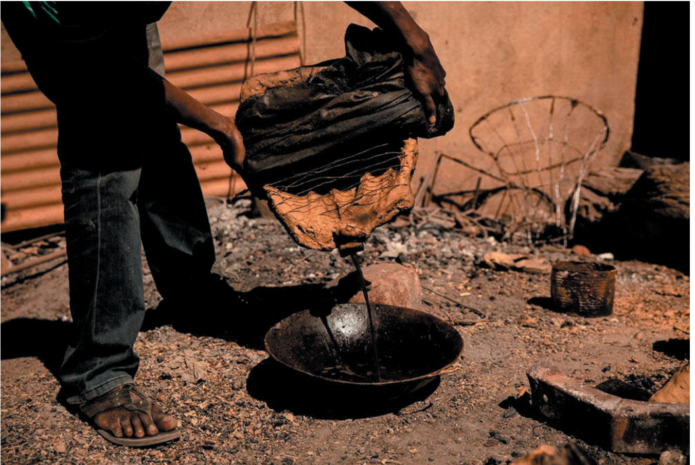
Top, a beeswax model of the lamp is wrapped in a mix of clay and horse dung, secured with metal wires, and baked for a few hours. Bottom, once the clay has hardened and the wax melted, metalsmith Alidou Zougrana drains the melted wax into a bowl, for reuse. Photography: Sophie Garcia
