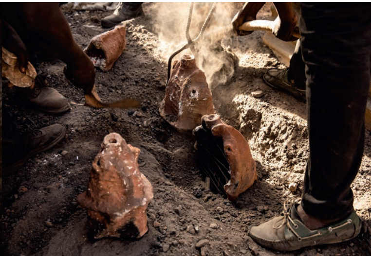
6. The metal is left to cool and harden in the clay moulds for about an hour and a half
